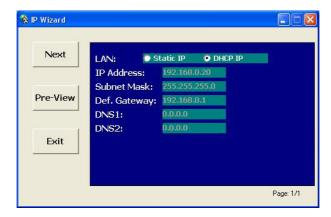
If no IP address is assigned after 30 seconds, ICA-525 will use its default address 192.168.0.20. User may open your web browser, and key in http://192.168.0.20 in the address field to login web configuration page and refer to our User's manual in the bundled CD disk to configure.
